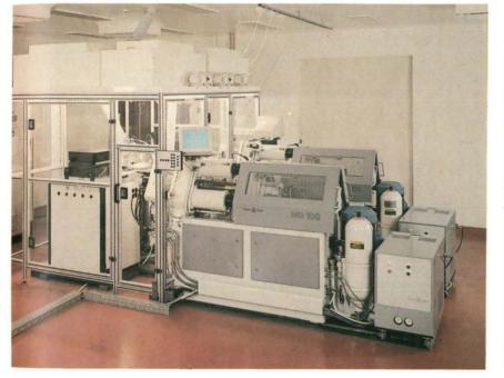
The Double Track system has a production capacity of up to 1000 discs per hour. Compact design and high output make it the ideal manufacturing unit for plants where space is at a premium.
